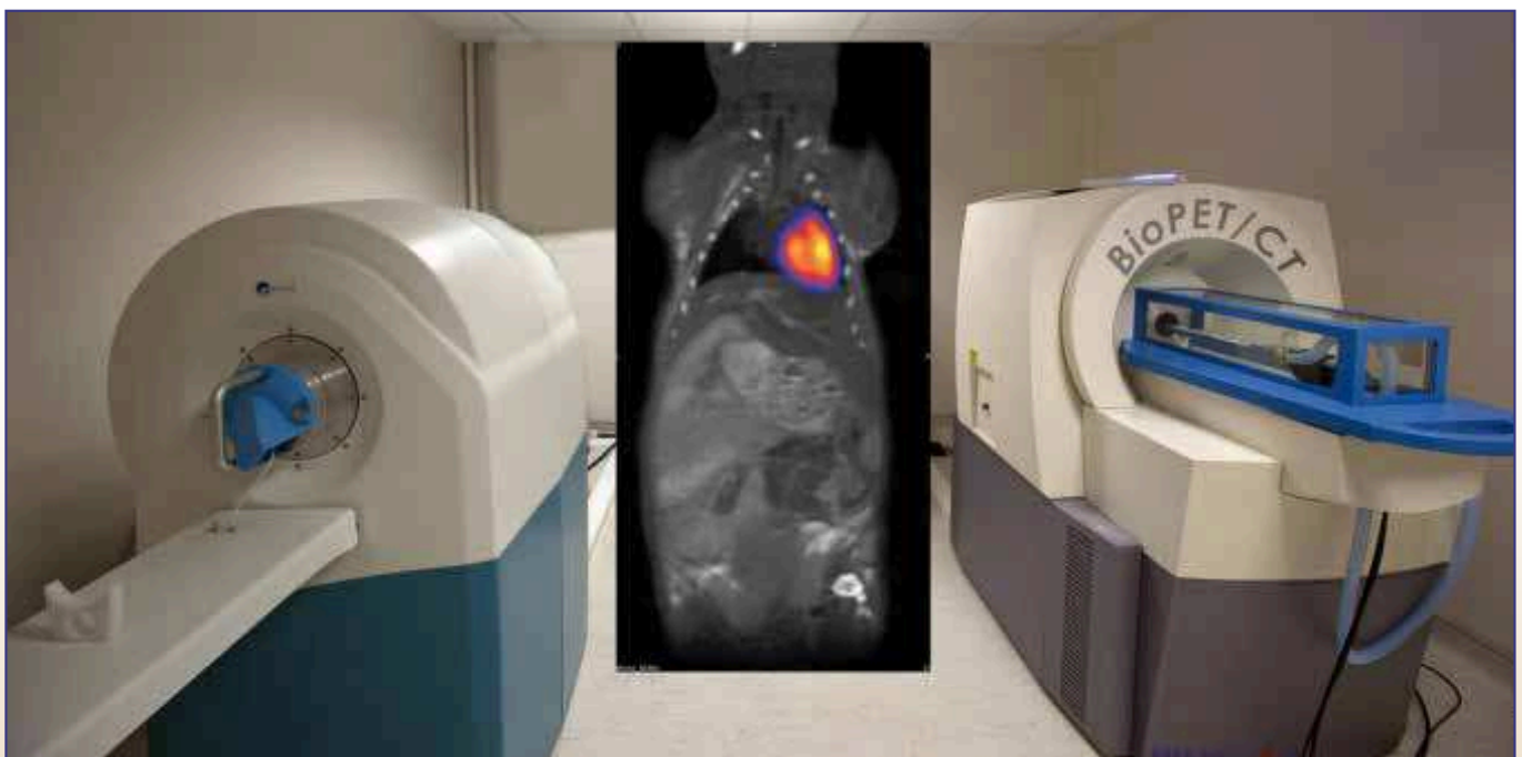
Figure 1. IMAPI Phase I: Two separate imaging systems installed in the preclinical imaging room. On the right, the PET/CT system with the universal animal handling cell and on the left the MRI 3.0T system with the identical animal cell completely inside the magnet bore.
