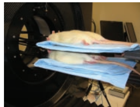
Figure 4. Multiple animal imaging in a large-bore small animal PET scanner, where 4 rats are scanned simultaneously in a 2x2 arrangement
